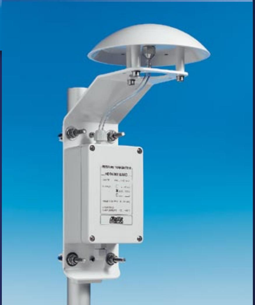
HD9408TR, is carried out through the HV55 special tube (inside Ø : 3mm, outside Ø : 6mm), which is resistant to climate changes and UV. Maintenance and cleaning are very simple. Plastic parts are in LURAN S777K, manufactured by BASF. It is strongly suggested to use non-aggressive cleaners, compatible with the plastic material.
